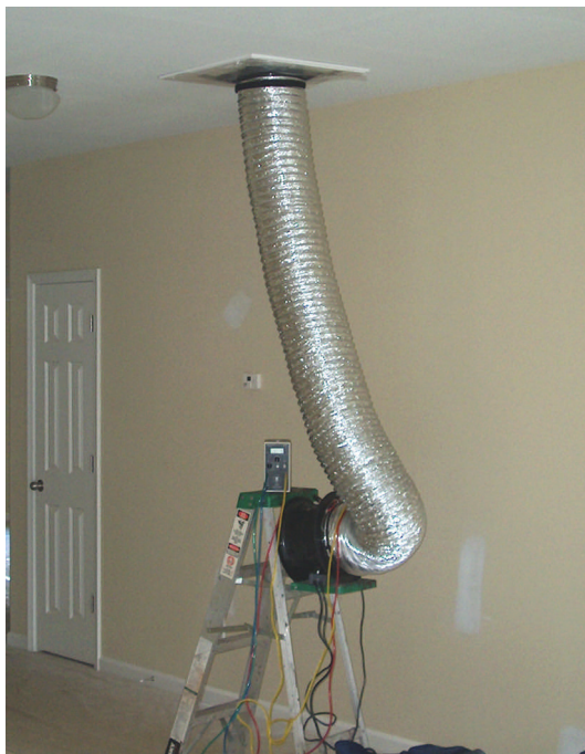
LEAKY DUCTS can be a significant source of energy loss in both new and existing homes. Duct tightness testing can help identify leaks. Photo: Kes Spray Insulation
